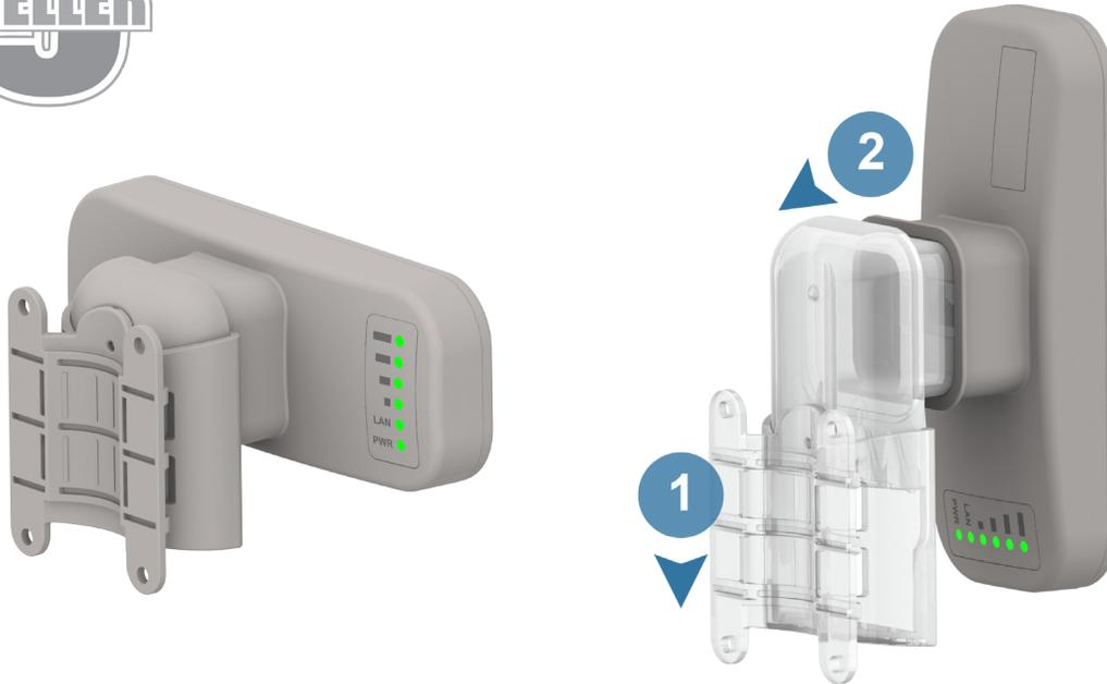
The APC Propeller 5 is a new generation wireless device designed for client and small scale base-station applications. It has a unique mechanism to do mechanical antenna parameter shifting and achieve the best performance in different operation modes (patent pending).
